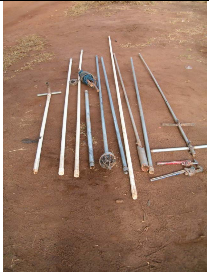
Plastic Threaded 1 1/4 inch PVC “Drill Stem” plus reamer, Auger and most of the material that you will need to drill.
